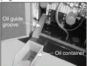
② Move the plastic rounded lid on the top of genset, unscrew the cylinder head oil cap, fill the oil until reach the oil gauge max limited (4.1. ②), in the end screw back the cylinder head stud.
