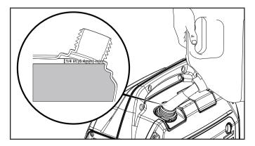
3. Screw on the gasoline cap and wipe away any spilled fuel.
