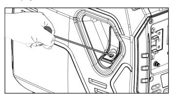
As the engine warms up, turn the dial to the gasoline "RUN" position.
