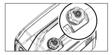
4. Turn the dial counterclockwise to the "STOP" position.
