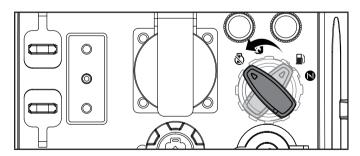
**Important:** Always ensure that the dial and fuel vent on the fuel cap are in the "OFF" position when the generator is not in use.
