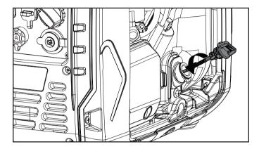
4. Tilt the generator on its side and allow the oil to drain completely.
