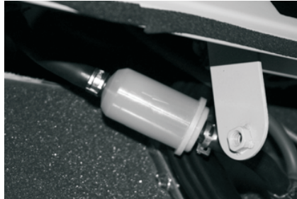
( Figure A – Change Fuel Filter located inside front access panel once a year )
