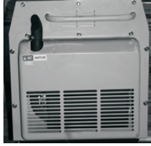
1. Remove Muffer Access Panel
