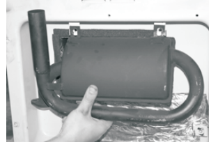
3. Remove Both Mufflers
