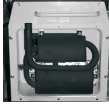
2. Remove Dual Muffer System
