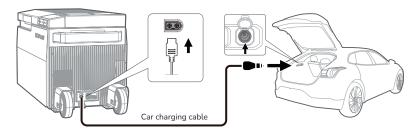
This product supports car charging through the  $12\,\text{V}/24\,\text{V}$  car charging port and charges the connected EFBX100-EB battery pack (optional) with a maximum current of 10 A.
