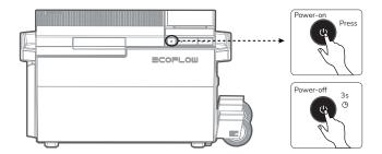
**Power-on:** Press the power button to turn on the device. The general power indicator becomes fixed.
