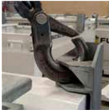
Galvanized stacking corner doubles up as a lifting bracket.
